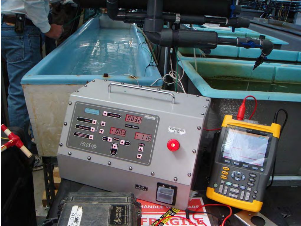
Figure 4. Midwest Lake Electrofishing Systems Infinity pulsator used for all electrofishing trials and Fluke scopemeter used to monitor frequencies, duty cycles and peak voltages
