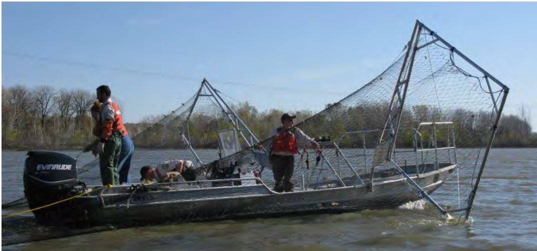
Figure 1. Paupier prototype I deployment in a Missouri River floodplain scour hole.
