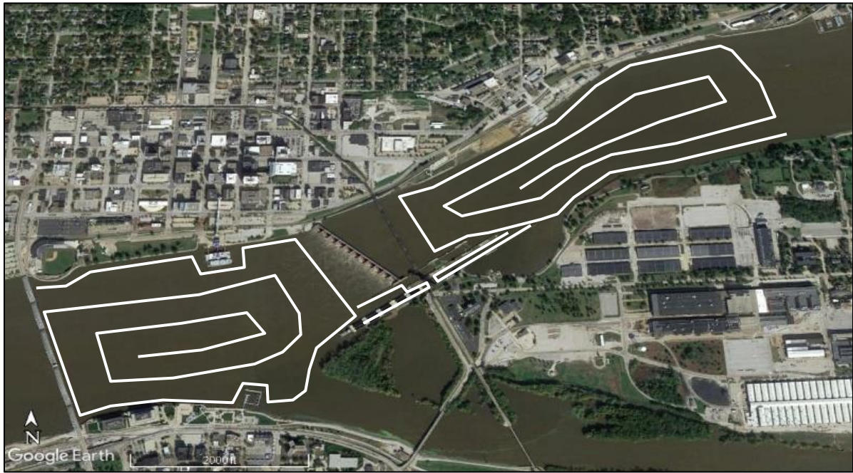
Figure 9. Generalized paths of hydroacoustic surveys conducted at Lock and Dam 15 of the UMR.
