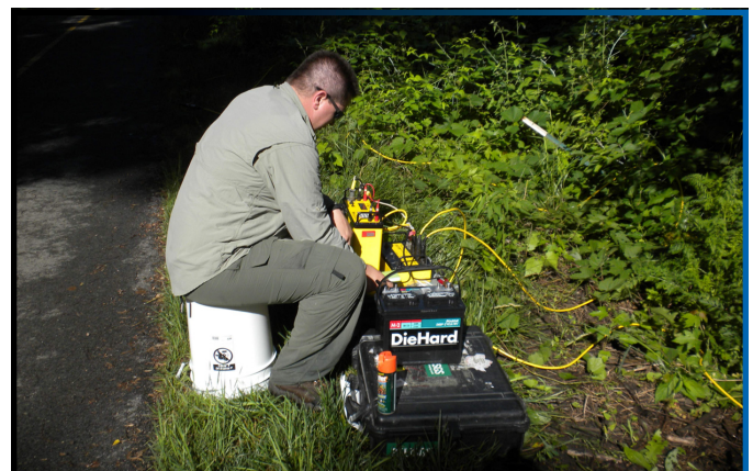
USGS hydrologist collecting resistivity data along the CSSC and the DPR. This data was compared to the MBES and water-quality data to optimize drilling locations, June 2010.
