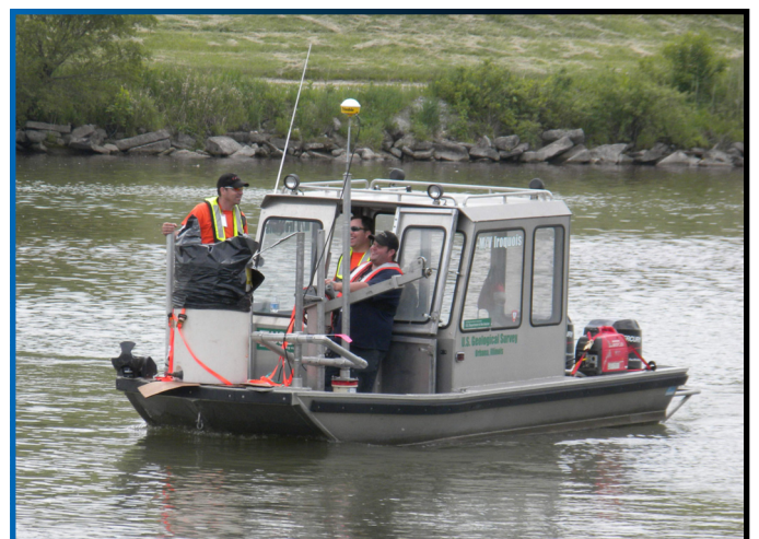
Rotenone Treatment near O'Brien Lock in May 2010: USGS boat with dye injection, water quality and ADCP equipment, with USGS hydrologists.
