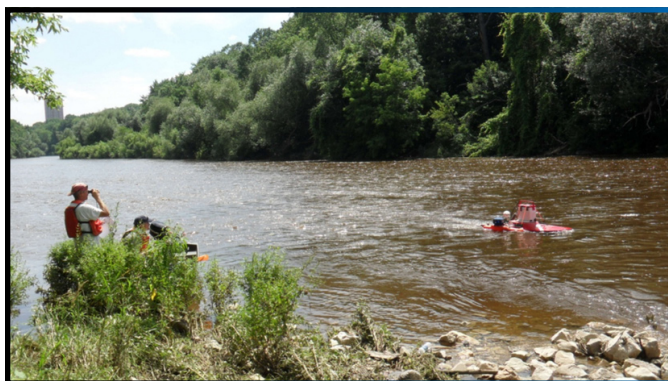
ADCP and water-quality data collection on the Milwaukee River in July 2010 with USGS hydrologists.
