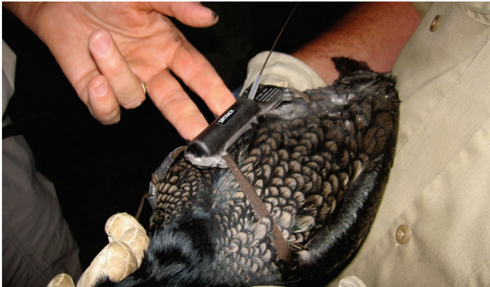
Figure 6. A Sirtrack Argos Satellite PPT transmitter is affixed to a Double-Crested Cormorant at the Baker's Lake colony site, May 2012.
