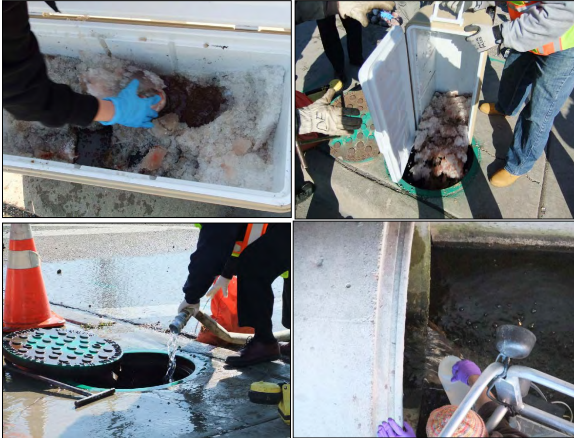
Figure 2.1. Storm sewer experiment trials (top row, left to right): Asian carp tissue chunks in ice (tissue removed prior to deposition in sewer); ice slurry deposited into sewer; (bottom row, left to right) fire hose used to flush system before and after slurry deposition; water collected from outflow at entrance to river from boat.
