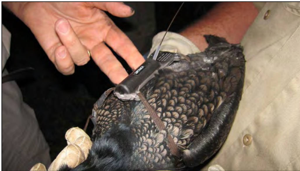
Figure 2.10. A Sirtrack Argos Satellite PPT transmitter is affixed to a double-crested cormorant at the Baker's Lake rookery site.
