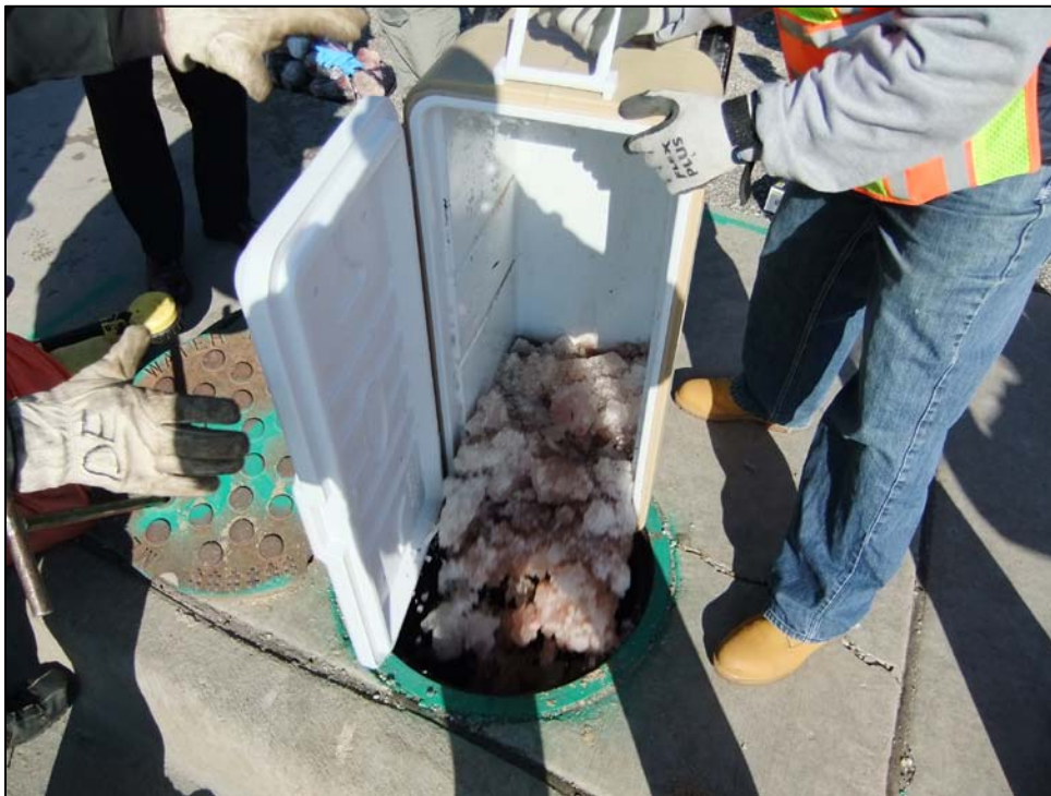
Exhibit 2. After sewer was flushed, fish pieces were removed from the cooler and the ice was dumped into sewer.
