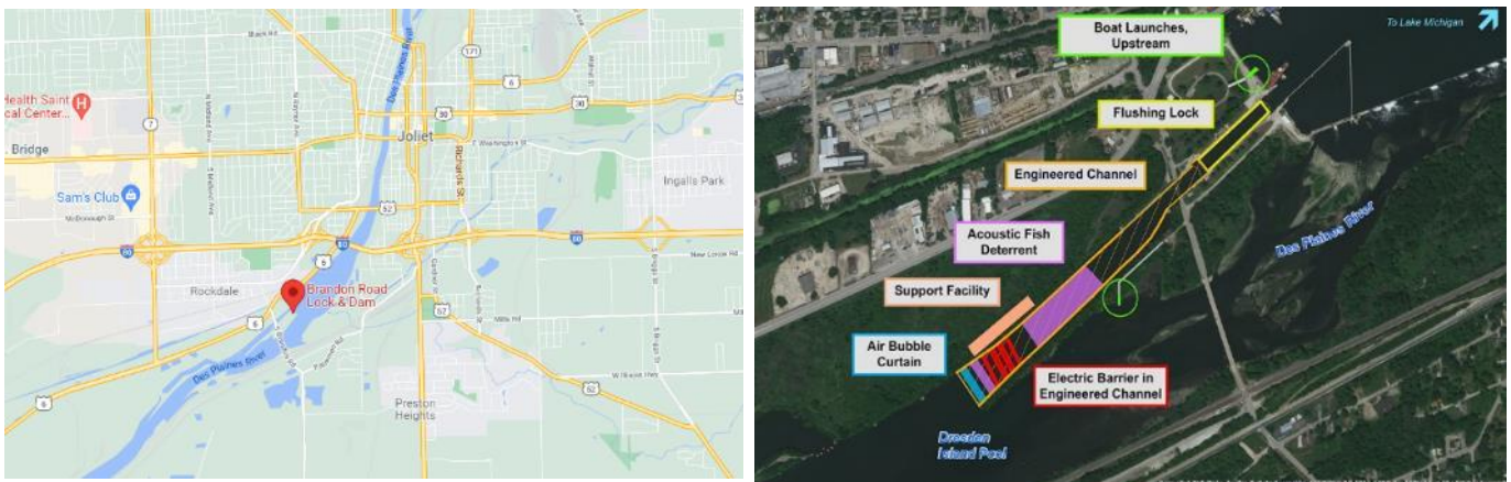
Figure 11. ( Left) Location of the Brandon Road Lock and Dam, Joliet, Illinois. (Right) Diagram of Multiple Deterrents Under Consideration for BRLD Interbasin Project Deployment (Photo from www.usace.army.mil/Media/News/NewsSearch/Article/2465911/glmris-brandon-road ).
