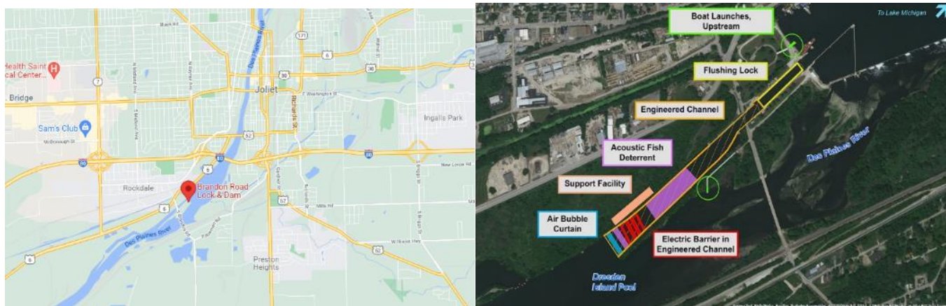
Figure 10. ( Left) Location of the Brandon Road Lock and Dam, Joliet, Illinois. ( Right) Diagram of Multiple Deterrents Under Consideration for BRLD Interbasin Project Deployment (Photo from www.usace.army.mil/Media/News/NewsSearch/Article/2465911/glmris-brandon-road ).
